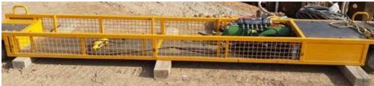
Figure 5: Breathing Air Cylinder and Manifold Securely Fastened to Electric Cart.
