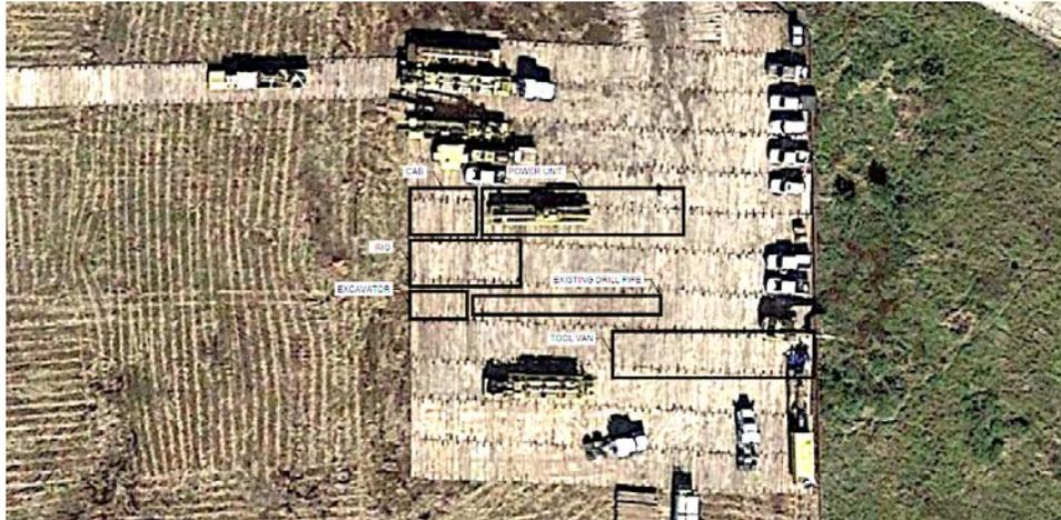
Figure 7: HDD Equipment Layout
