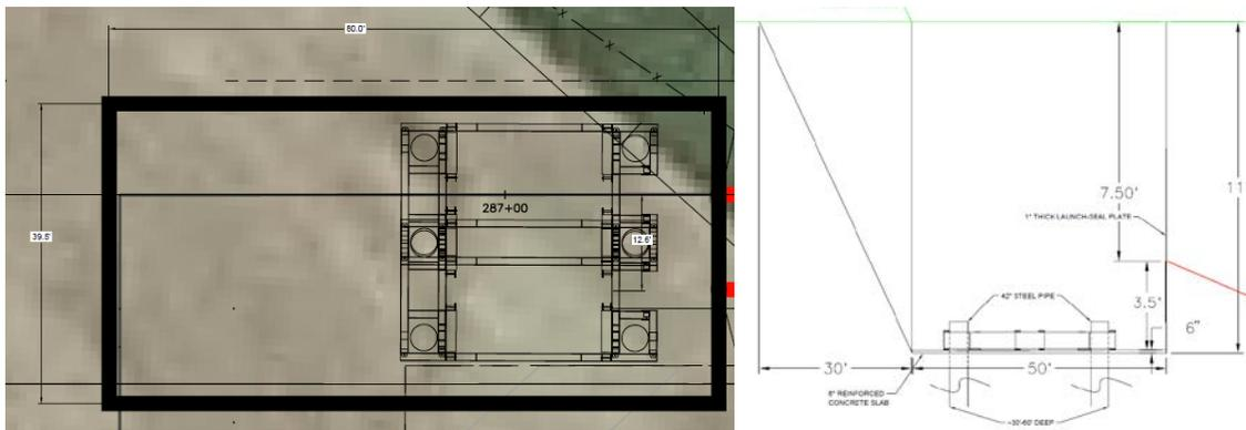
Figure 4: Direct Pipe® Pit and Foundation Design
