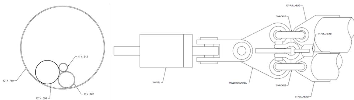
Figure 8: (a) Conduit Bundle Cross Section and (b) Pulling Assembly
