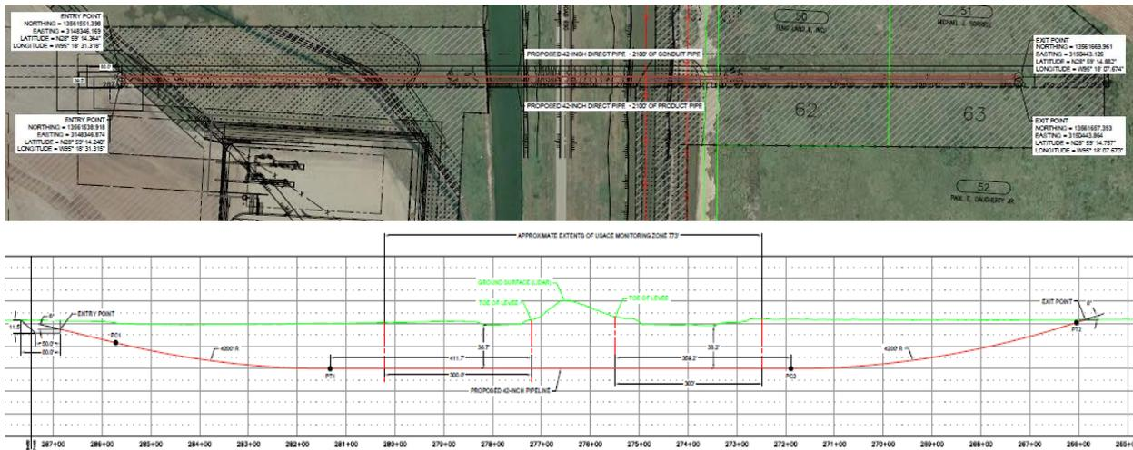
Figure 1: Drill Layout and Profile (not to scale)
